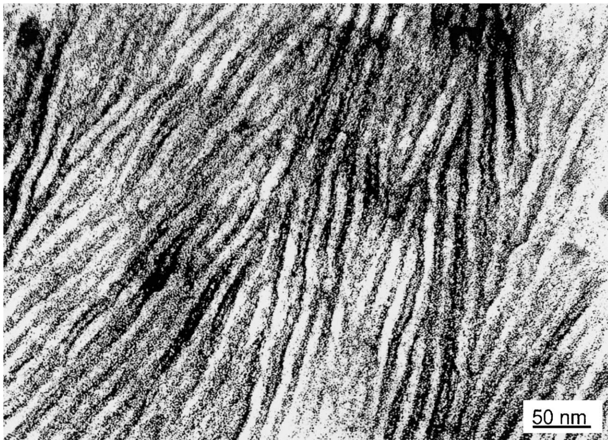
Figure 3 TEM micrograph showing in detail the morphology of \beta -iPP; RuO 4 staining causes the less denser amorphous phase to appear dark.
